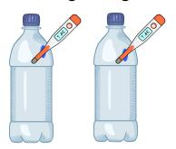
Step 2: Fill each bottle 1/3 full of water, and insert the thermometer into the newly made hole, sealing around the edges with blu-tac.
